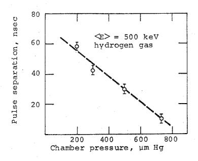
Figure 1 Proton pulse separation versus pressure.
